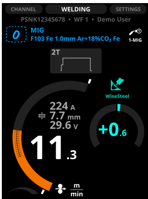
Figure 12: Raster pattern in the wire feed arc
