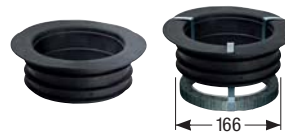
Quick-Fit the passage seal for core drillings, for Ecoguss / Practicus drain bodies with vertical outlet • with fire protection 1) 48 990 with approval Z-19.17-1719 • without fire protection 48 991
